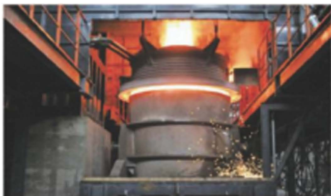
20-ton LF furnace
