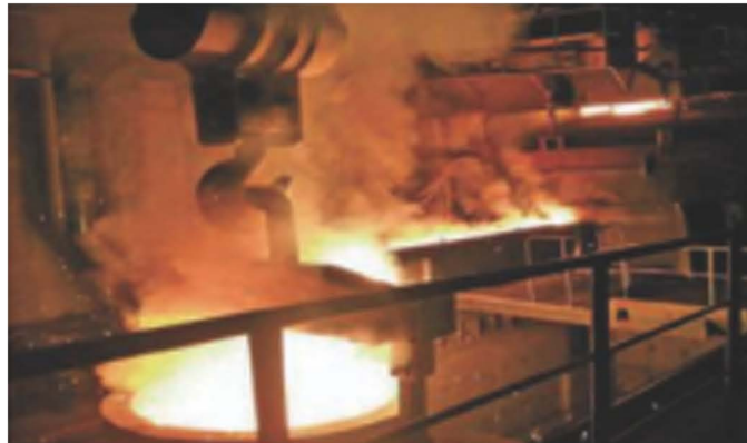
20-ton of purification furnace
