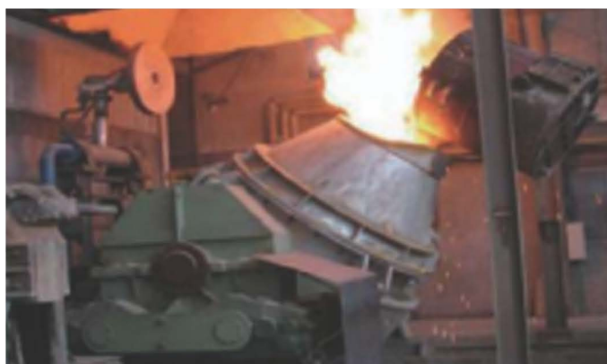
20-ton AOD refining furnace
